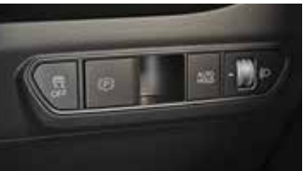
ESC (Electronic Stability Control)
