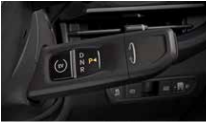
Shift-by-Wire (SBW) - Column Type
