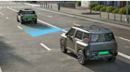
Leading Vehicle Departure Alert (LVDA)
